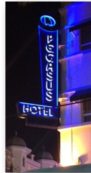
501 SOUTHARD STREET. REPLICA OF A 1940'S NEON SIGN USING LED HALO EFFECT INSTEAD OF NEON.
